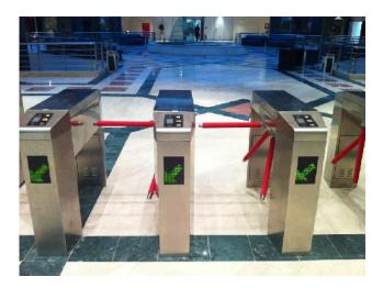
Semi-automatic electro-mechanical tripod turnstile consisting of casing, magnetic force turn plate, reader module, main controller module, direction guide, limit switch etc. for use at entrances to restricted / controlled zones.
